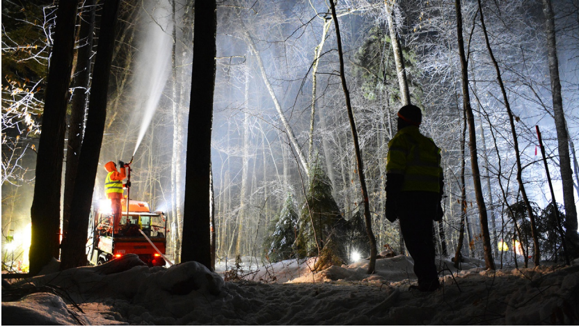
Fig. 6.12 Canopy icing in progress at Hubbard Brook for the Hubbard Brook Icing Experiment. Treatment plots were targeted by spraying water over the 15–20 m tall forest canopy from below. The falling water froze on contact with branches at air temperatures ranging from -14 to -9^{\circ}\text{C} . (Photo credit: Lindsey Rustad).
