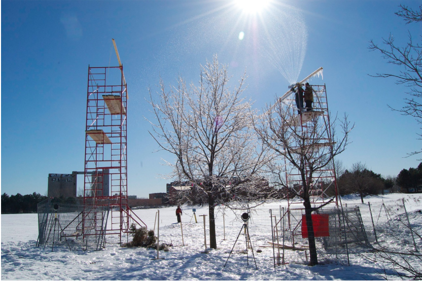
Fig. 6.10 Experimental icing in progress in February 2011 in Montréal, Québec, Canada. At center is a Norway maple that is 9 m tall with an approximate crown diameter of 5 m. Also visible are wooden dowels for measuring R_{eq} placed just beyond the drip line of the crown as well as underneath the crown.
